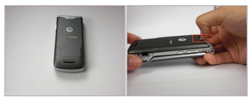
• Push down on the silver tab located at the top center of the back of the Motorola K1m cellphone.
