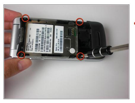
Detach battery dock by removing the 4 black screws on each corner of the phone with a T5 Torx Screwdriver.
