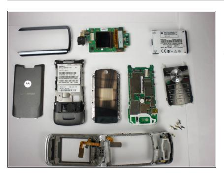
The final result should look similar to this layout of the disassembled Motorola K1m.
