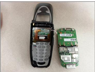
• Remove the motherboard by firmly grasping the edges of the circuit board with one hand and the phone with the other and pulling up on the motherboard slightly and then pulling it straight down toward the bottom of the phone.
