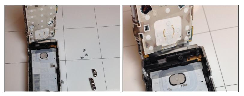
• Remove the back, being careful not to detach the motherboard from the back and to not pull them fully out (both attached at the upper left corner by a black strip).
