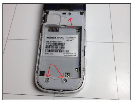
• Red arrows indicate which screws must be removed in order to get to the motherboard.
