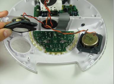
Remove the eight 11mm Phillips #1 screws that connect the speakers to the white outer case.
