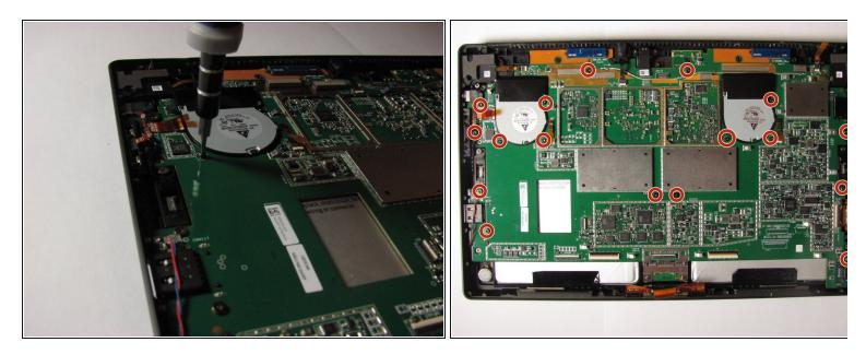
• Unscrew the 17 T5 torx screws on the mother board with the T5 torx screw driver
