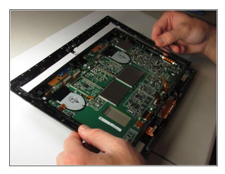
• Lift the screen bezel from the Surface Pro.
