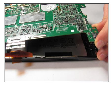
Once all screws are removed, gently lift up the logic board with your hands to pull it out.
