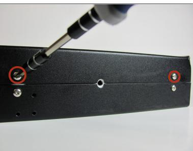
Unscrew the top four 6.0mm Phillips head screws counterclockwise on the left and right side of the device using a #1 Phillips head screwdriver.
