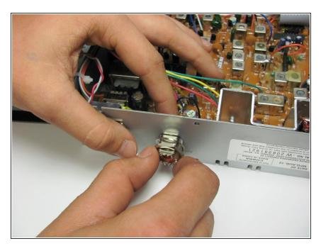
Remove the securing nut and washer from the antenna connector.
