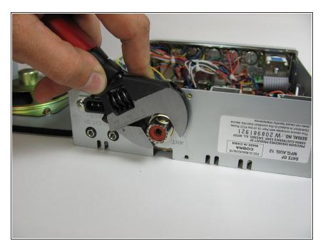
Use a wrench to unscrew the nut counterclockwise, that secures the antenna connector to the device.
