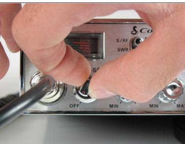
Turn the power switch, the leftmost knob, counterclockwise to off.
