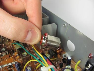
Gently pull the antenna connector through its hole into the case.
