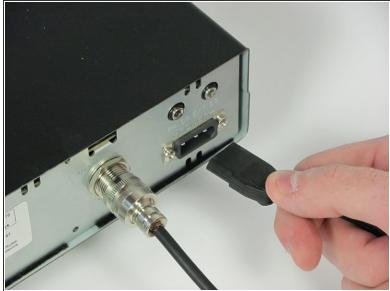
Turn the device around and firmly pull the power cable plug to remove it from the radio.
