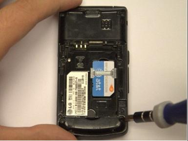
• Use a small Phillips head screwdriver to remove the six 3mm screws identified in the photo.
