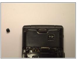
Using a spudger or other sharp tool, remove the two rubber pieces on the top of the back of the phone.
