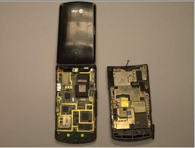
• Use tweezers to carefully unplug the wires connecting the speakers to the mother board.
