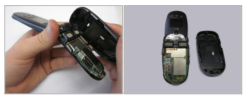
• Remove the back cover completely from the phone.
