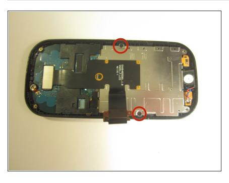
Use a screwdriver and corresponding bit to remove the two 1mm screws. Set the screws aside.
