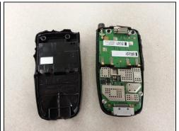
• Starting from the bottom and working towards the top, use a spudger to pry the back cover off the phone.
