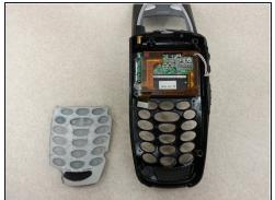
• Using your fingers, carefully lift the rubber keypad from the phone.
