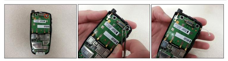
Using a pair of <u>tweezers</u>, firmly grasp the connector at the top of the phone and pull the connector straight away from the phone.
