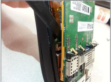
• Unclip the ribbon cable, located underneath the motherboard, by using the spudger to push up on the dark brown part of the connector located on the circuit board.
