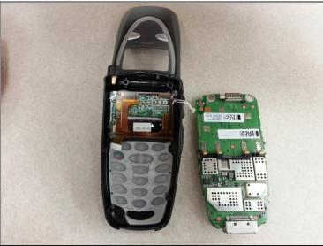
• Remove the motherboard by firmly grasping the edges of the circuit board with one hand and the phone with the other and pulling up on the motherboard slightly and then pulling it straight down toward the bottom of the phone.
