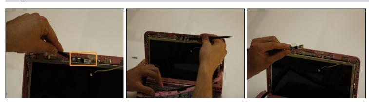
Use the spudger to pry each side of the webcam until it releases from its adhesive back.
