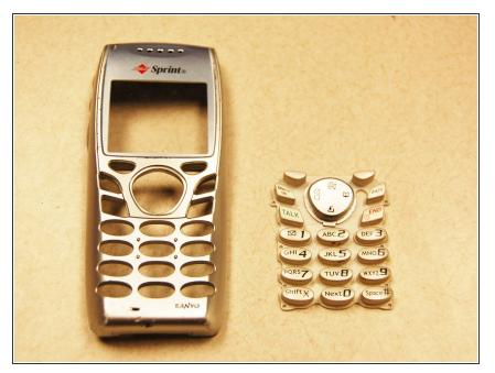
• The plastic keys are attached to the back side of the front case. To remove the keys, pull the plastic piece out of the front case using the plastic opening tool.
