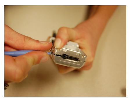
Use the plastic opening tool and slide it around the phone to pull apart the front and back casing.
