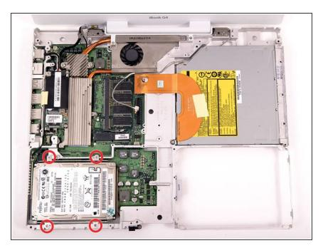
Remove the four Phillips screws securing the hard drive to the metal framework.
