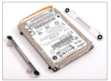
Remove the hard drive brackets from the left and right sides of the hard drive.
