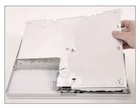
• Lift the bottom shield off.
