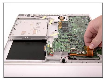
Turn the computer over and disconnect the orange hard drive cable, removing tape as necessary.
