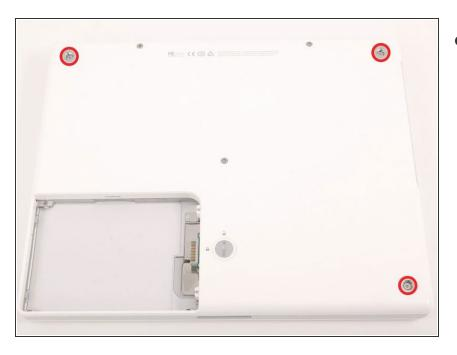
Remove the three newly-revealed Phillips screws.
