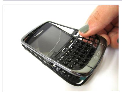
• Lift and remove the frame.
