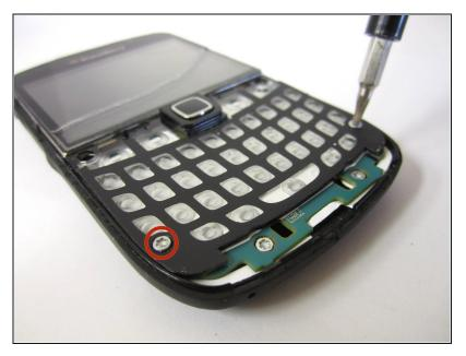
Locate and remove the two 5mm screws on top of the keyboard base with a T6 Torx screwdriver.
