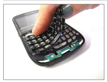
• Lift and remove the keyboard.
