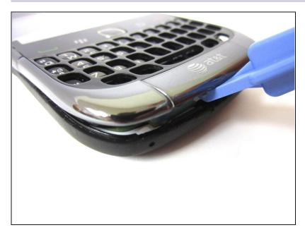
Use a plastic opening tool to lift the bottom edge of the front cover.
