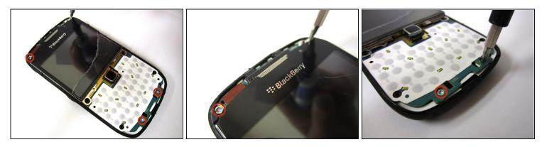
• Remove the four 5mm screws on the top and bottom of phone with a T6 Torx screwdriver
