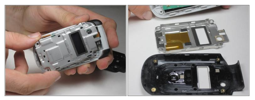
• After removing the external casing, there are no more screws holding on the gray metal plate. Carefully separate the gray plate from the rest of the phone by simply lifting it off.
