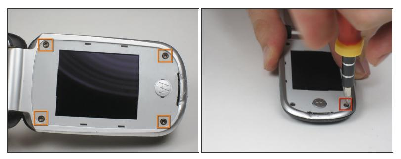
• Unscrew the four screws using the T6 Torx Screwdriver.
