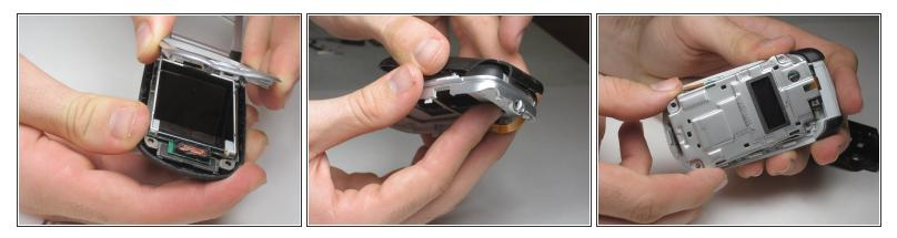
Peel back the screen protector frame. Close phone at the hinge, then pull off the front outer casing.
