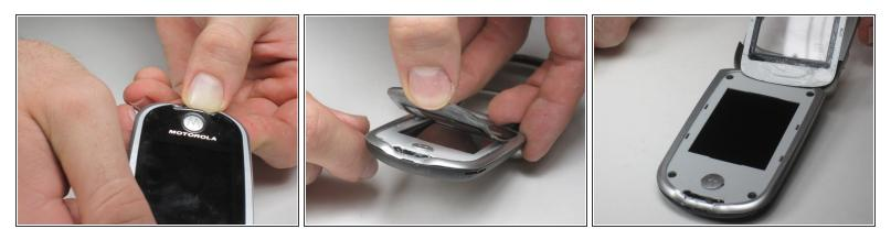
• Using your thumbnail or a thin flat head screwdriver, peel back the screen protector on the inside of the phone: It is only held on by glue but may take a good amount of force to be removed.
