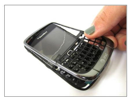
Lift and remove the frame.
