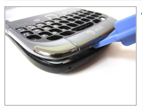
Use a plastic opening tool to lift the bottom edge of the front cover.
