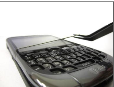
Place the phone face up and use tweezers to securely grip and lift the screen upwards.
