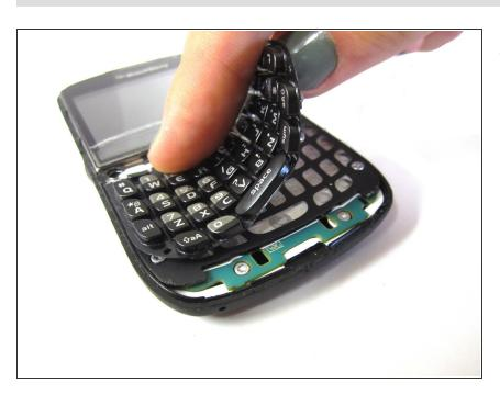
Lift and remove the keyboard.
