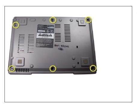
Flip over the PlayStation and remove the six screws from the bottom.
