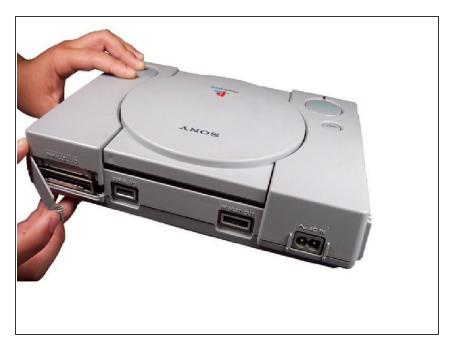
Remove the parallel port cover on the back of the PlayStation
