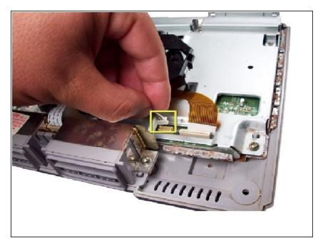
Disconnect the second cable by pulling up on the plastic connector at the end.
