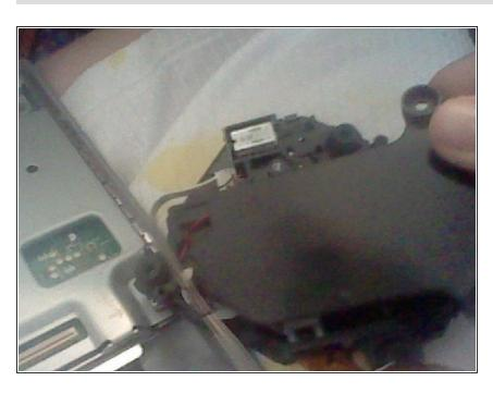
Take the bottom piece you took out and place it on the new Optical drive and screw it on the new drive.
