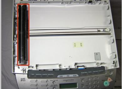
Remove the black component by gently pulling it up from the black scanner belt
