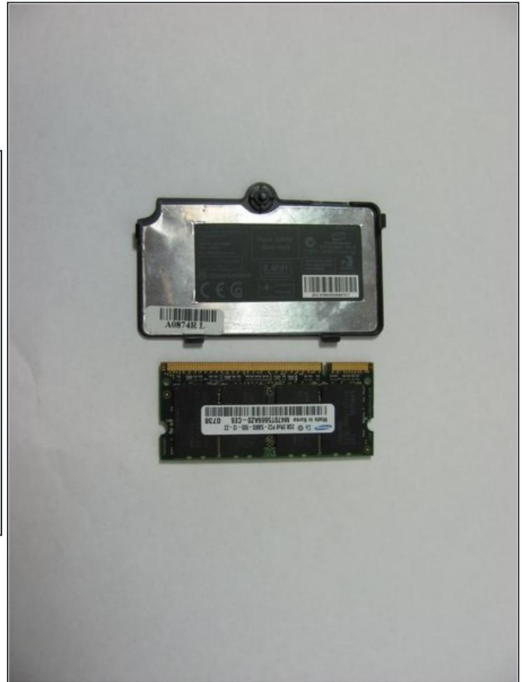
**⚠** The RAM chip is susceptible to static electricity. Before grabbing the RAM chip, make sure you have discharged the electricity from your hands by touching a metal surface other than your computer.
