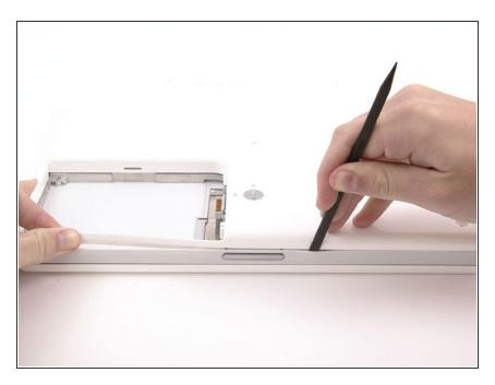
Run a spudger along the seam between the lower case and upper case on the front of the computer to free the tabs locking the lower case.
