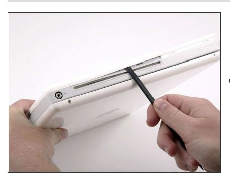
There are three tabs over the optical drive that must be released before the lower case can come off. Slide the spudger into the lower case above the optical drive and run it toward the back of the computer until you hear three distinct clicks.
