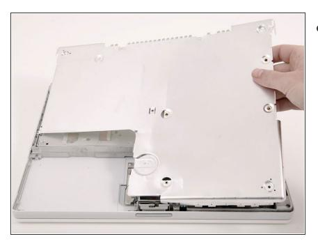
Lift the bottom shield off.
