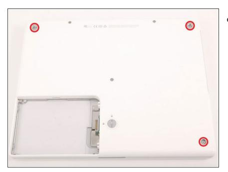
Remove the three newly-revealed Phillips screws.
