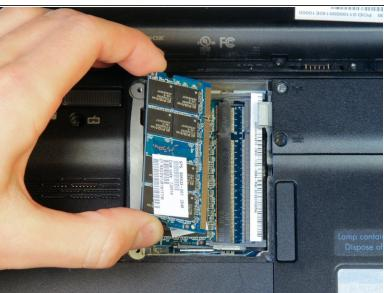
Using one hand, pull the RAM up and to the left to remove it.
