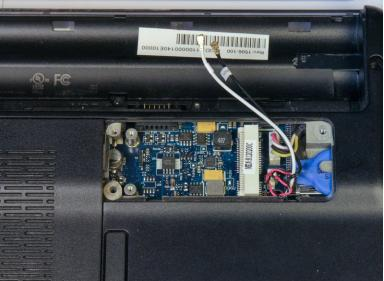
Grab the sides of the wireless card and pull it up and to the left to disconnect from the laptop.
