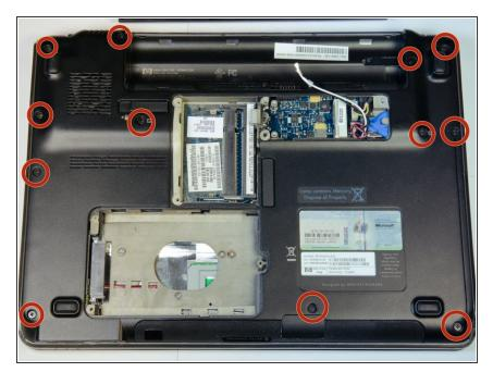
Locate and remove all 12 black screws on the back cover. They have a 3.5 mm diameter head and are 13 mm in length.
