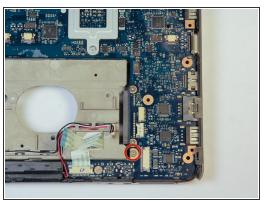
Locate and unscrew the three, silver, 3.5mm diameter head, 3mm long screws on the motherboard.
