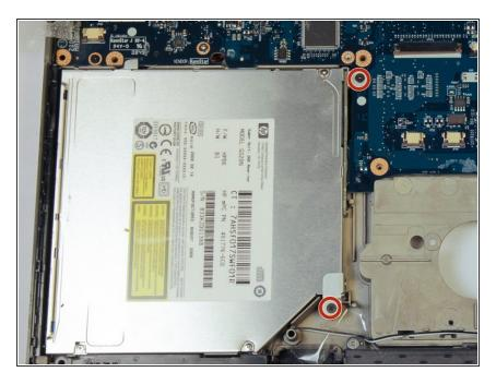
Locate and remove the two black longscrews holding the CD drive.
