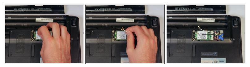
• Using your hand, pull the black and white antenna wires upwards.
