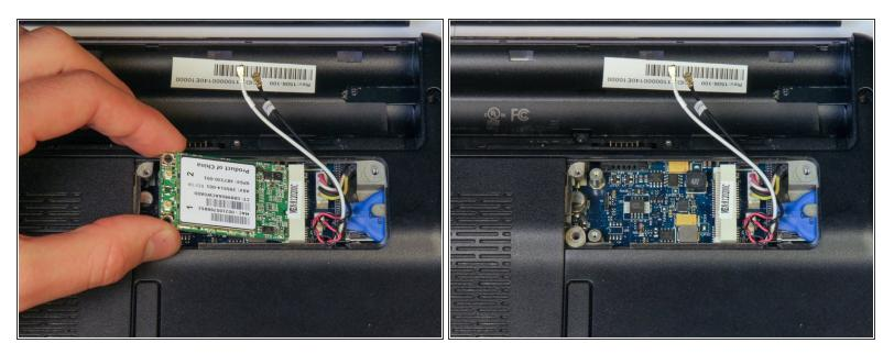
• Grab the sides of the wireless card and pull it up and to the left to disconnect from the laptop.
