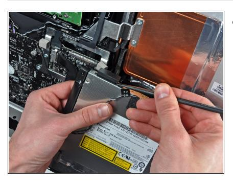
Use the flat end of a spudger to help disconnect the optical drive cable.
