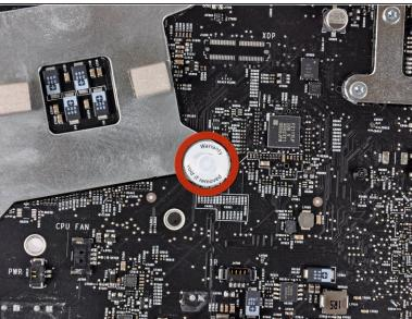
(i) If present, remove the "Warranty void if removed" stickers covering one screw on either side of the heat sink.
