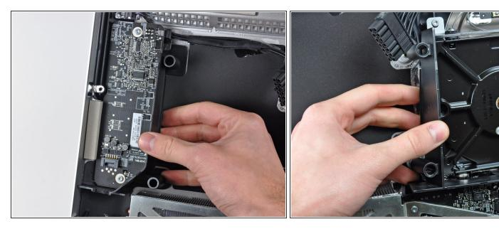
Remove the plastic ducts from the side of the LED driver board and the hard drive by pulling them away from the outer case.
