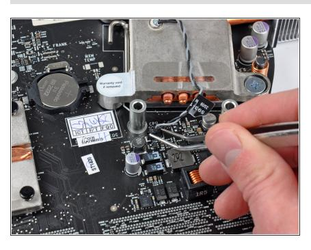
Use a pair of tweezers to lift the heat sink thermal sensor connector straight up out of its socket on the logic board.
