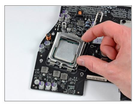
Rotate the CPU clamp away from the CPU.
