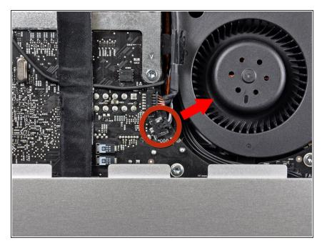
Pull the optical drive thermal sensor connector straight away from its socket on the logic board.
