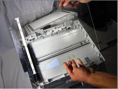
After you have taken off the plate, check to make sure that there is no broken glass. If there is broken glass handle it with gloves. Broken glass, if handled improperly, can cause physical injury.
