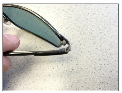
• The problem at hand: The screw will not fit through the arm because a spring is pulling on the hinge (and screw hole) in the arm.
