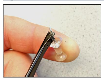
Insert a pushpin through the hole and use it as leverage to extend the spring hinge outwards.
