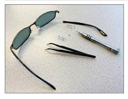
• These are the tools I used to insert the screw through the spring hinge. In the video a paperclip was used, but the paperclip I had on-hand could not fit into the tiny recess in order to jam the spring open.
