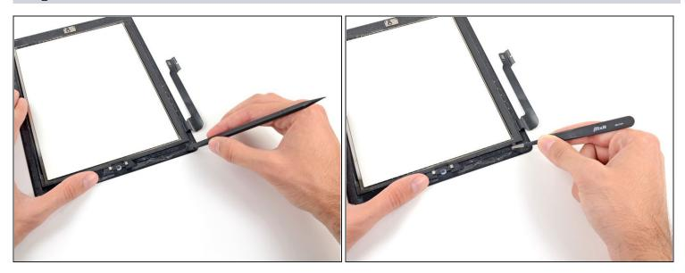
• Use the flat edge of a spudger to scrape the old adhesive off the bottom right corner of the front panel assembly.
