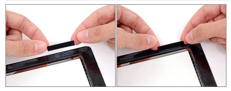
• Place the short rectangular shaped adhesive strip on the top left side of the front panel.
