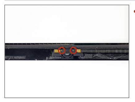
Remove the two 2.1 mm Phillips #00 Phillips screws securing the home button control board to the home button mounting bracket.
