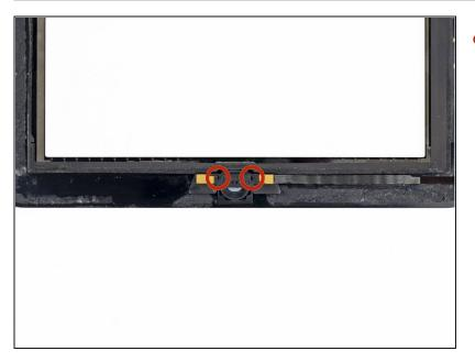
Insert the two 2.1 mm Phillips #00 Phillips screws back into the home button control board to secure it against the home button mounting bracket.
