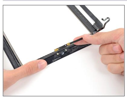
Lift and remove the home button control board up off the home button mounting bracket.
