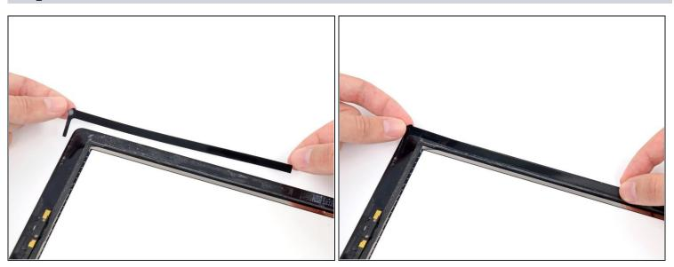
• Place the long L-shaped adhesive strip on the bottom left corner of the front panel.
