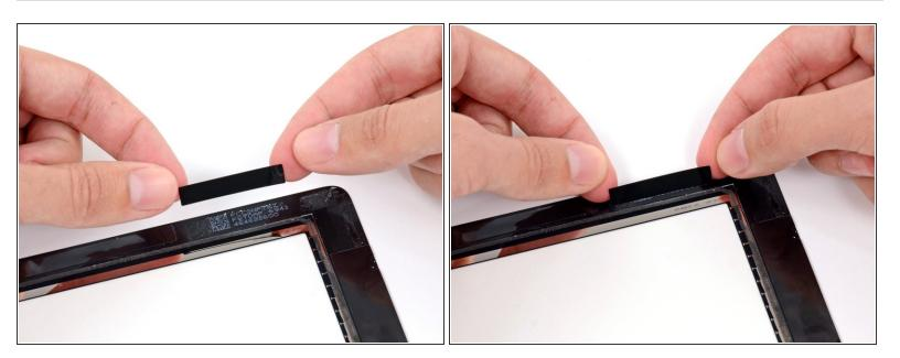
Place the short rectangular shaped adhesive strip on the top left side of the front panel.
