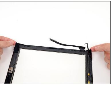
▶ Place the elongated C shaped adhesive strip on the right side of the front panel.
