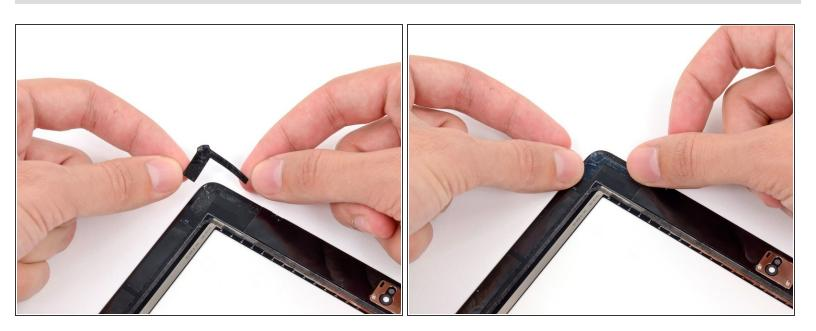
Place the last, short L-shaped adhesive strip on the top left corner of the front panel.
