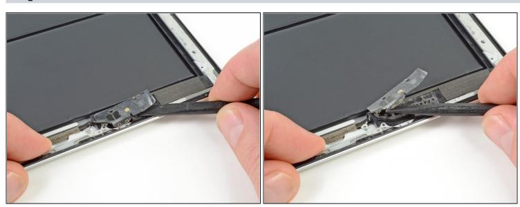
• Use the flat end of a spudger to loosen the foam adhesive holding the Wi-FI antenna to the speaker assembly.
