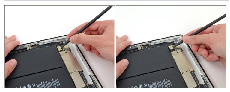
• Use the flat end of a spudger to pry the Lightning connector cable straight up out of its socket on the logic board.
