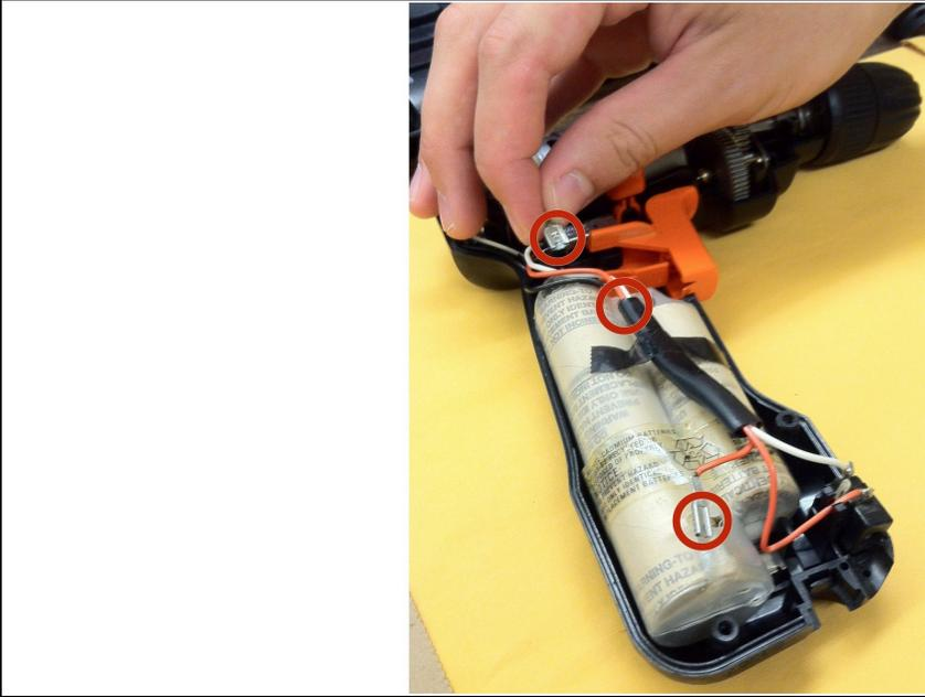
**⚠ SHOCK WARNING:** Ensure wire ends do NOT touch each other! Disconnect the battery from the drill by pulling out the 3 terminals.
