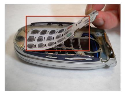
Peel the white keypad off the casing.
