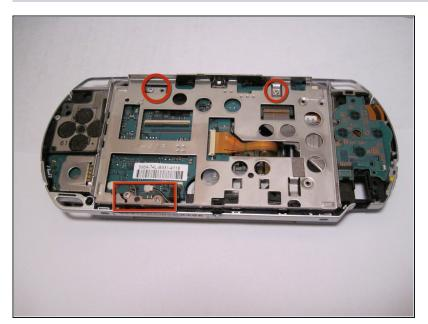
Remove the screws on the top and bottom of the frame. Be sure to keep track of where you took each screw out of.
