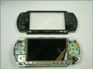
• Gently separate the outer plastic casing from the rest of the system as shown.
