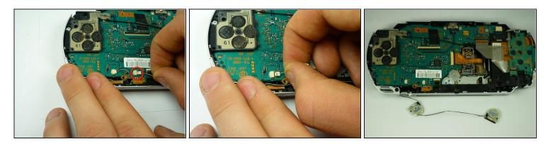
Gently unplug the speakers from the socket. The speakers are completely detatched when they are unplugged from the logic board.
