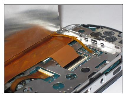
The LCD screen is still attached with ribbon cables. Gently lift up the LCD screen so you do not break them.
