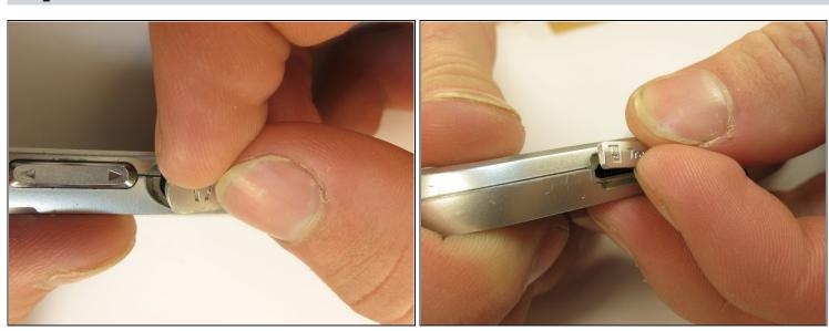
Pull open the earphone tab and the Trans Flash tab using your fingers.
