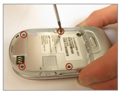
• Remove the four Phillips #00 screws underneath the battery.
