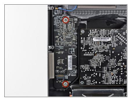
Remove the two 9 mm T10 Torx screws securing the LED driver board to the outer case.
