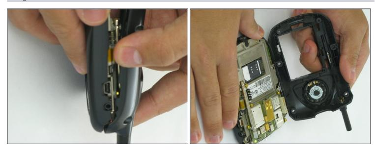
Slide the rear panel forward to reveal the motherboard.
