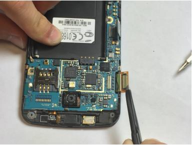
Disconnect the two ribbon cables from the motherboard.
