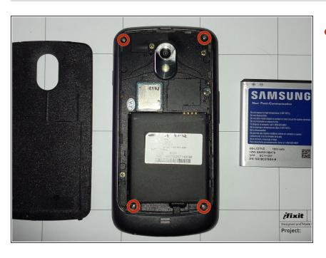
Remove the four 4.5 mm Phillips screws from the rear of the phone.
