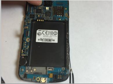
• Using tweezers, gently disconnect the antenna cable from its socket on the motherboard.
