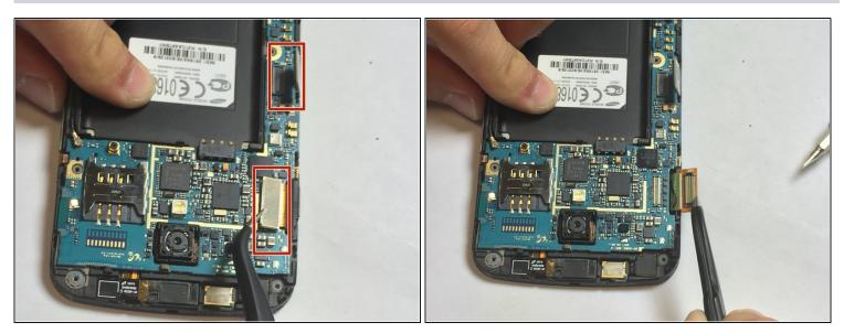
• Disconnect the two ribbon cables from the motherboard.
