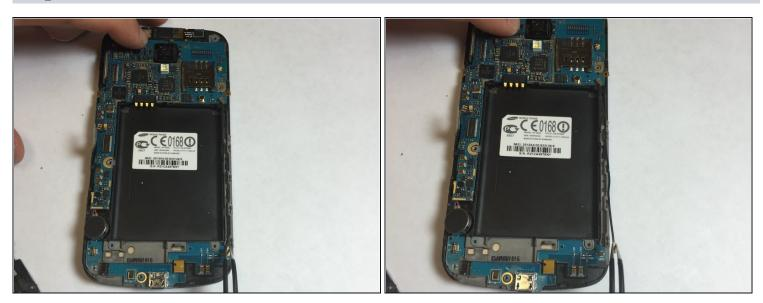
• Using tweezers, gently disconnect the antenna cable from its socket on the motherboard.
