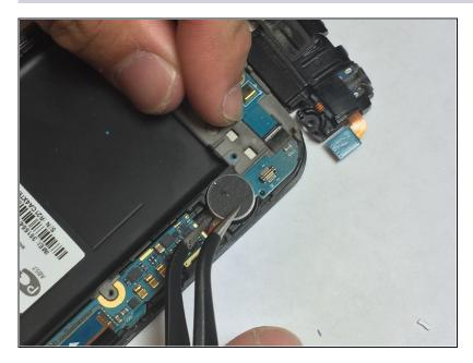
• Using <u>tweezers</u> or a spudger, lift the vibrator motor from its recess in the midframe.
