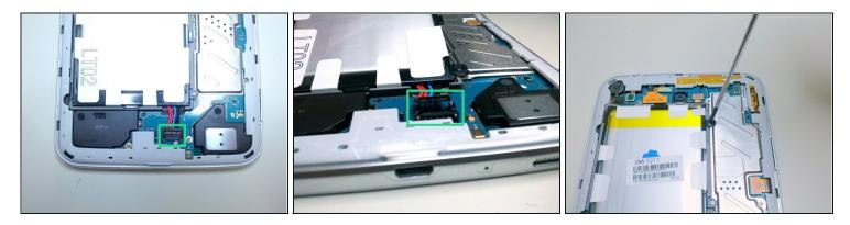
Once the back cover has been detached, you might want to detach the battery first to lighten the Tab's body when flipping around
