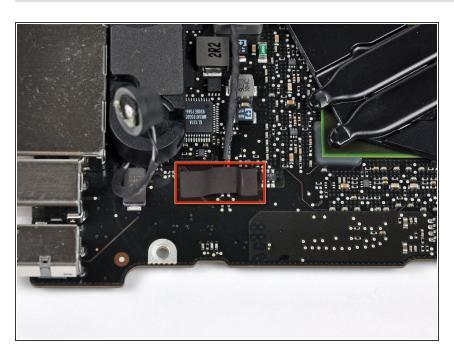
Remove the small strip of tape covering the left speaker connector.
