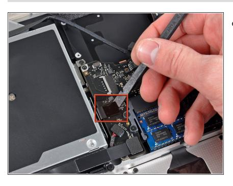
Use the flat end of a spudger to pry the optical drive cable connector up off the logic board.
