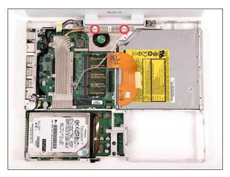
Remove the two Phillips screws from the white plastic fingers of the hinge grill.
