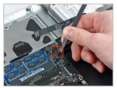
Using the flat end of a spudger, pry the subwoofer/right speaker connector straight up off the logic board.
