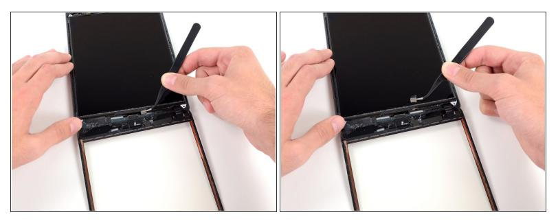
Use a pair of tweezers to peel up the small piece of tape connecting the LCD frame to the right speaker.
