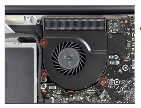
Remove three T6 Torx screws securing the right fan to the logic board and upper case.
