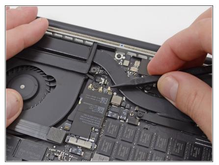
• Use the tip of a spudger to detach the three antenna connectors up from their sockets on the AirPort board.
