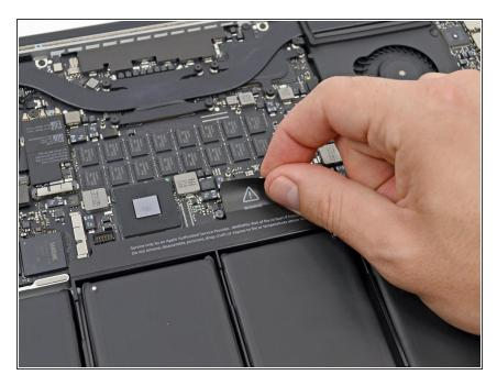
• Peel back the warning label covering the battery connector.
