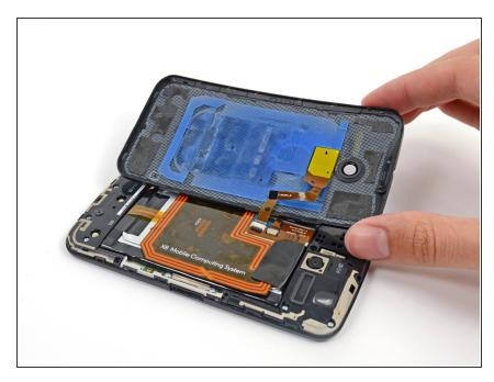
Gently set the back cover down in a way that exposes the camera flash cable connector, but does not put strain on it.
