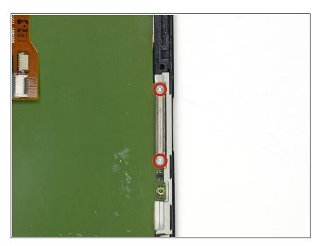
Remove the final two 3 mm T3 Torx screws from the SIM slot bracket.
