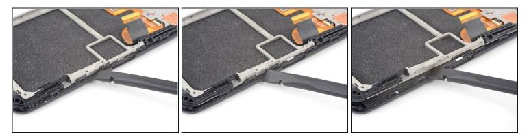
Use the flat end of a spudger to pry up the white mid-frame from the display assembly.
