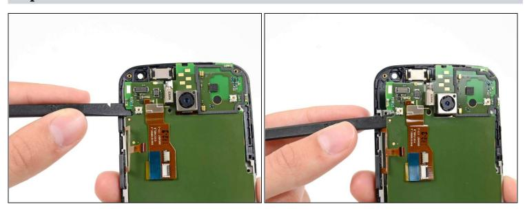
• Insert the flat end of a spudger under the motherboard above the button assembly cable, and pry it out of the phone.
