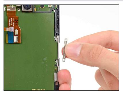
• Remove the SIM slot bracket from the motherboard.
