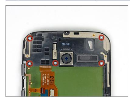
Remove the five 3 mm T3 Torx screws from the headphone jack/speaker assembly.
