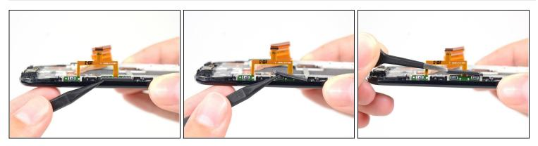
• Use the tip of a spudger to push the volume rocker button cover out of the display assembly, and remove.
