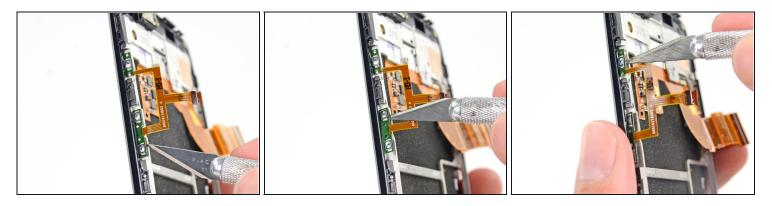
• Use the tip of a hobby knife or plastic opening tool to pry the button assembly off of the adhesive securing it to the display assembly.
