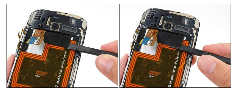
• Use the flat end of a spudger to peel the adhesive pull-tab off the top of battery.
