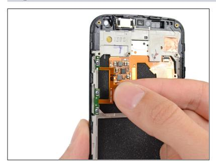
• Remove the button assembly cable from the display assembly.
