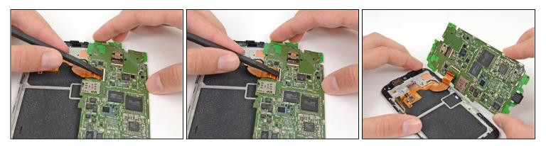
(i) Lay the motherboard down to allow access to the display cable connector.
