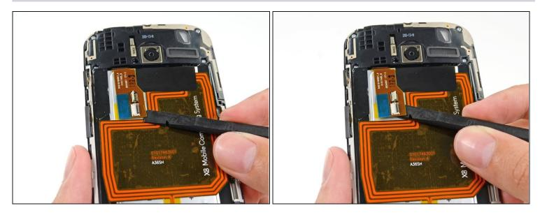
• Insert the flat end of a spudger under the interconnect cable to free it from the adhesive holding it to the battery.
