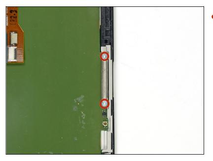
Remove the final two 3 mm T3 Torx screws from the SIM slot bracket.
