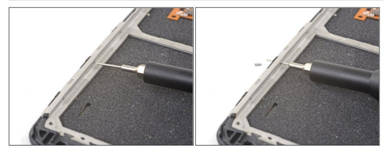
• Use a SIM eject tool, SIM eject bit, or a bent paper clip to gently push the pin outwards from within the case.
