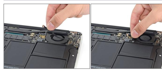
• Peel the iSight camera cable up off the adhesive securing it to the fan.
