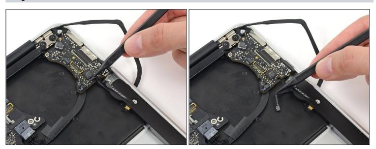
• De-route the cable from its notch in the I/O board.
