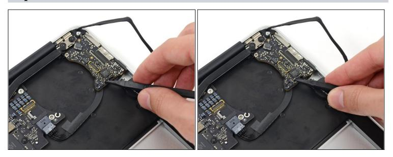
• Use the tip of a spudger to pry under the speaker cable near the connector to lift the connector straight up out of its socket.
