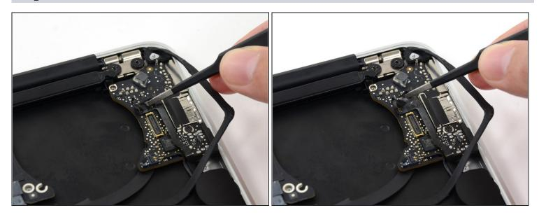
(i) If necessary, use <u>tweezers</u> to remove any tape covering the microphone cable ZIF connector.
