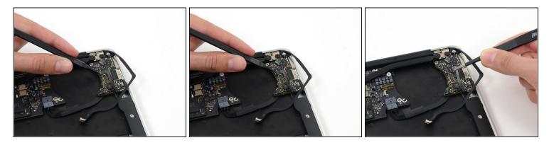
• Use the tip of a spudger to carefully flip up the retaining flap on the microphone cable ZIF socket.
