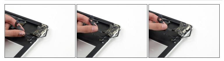
• Carefully lift the I/O board by its power cable and pull it away from the edge of the case.
