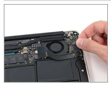
• Lift and remove the I/O board cable.
