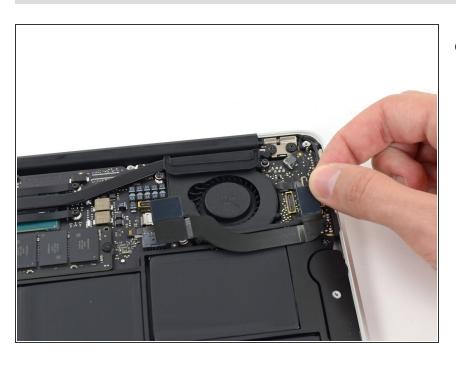
Lift and remove the I/O board cable.
