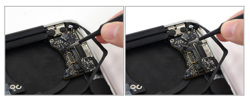
if necessary, use tweezers to remove any tape covering the microphone cable ZIF connector.
