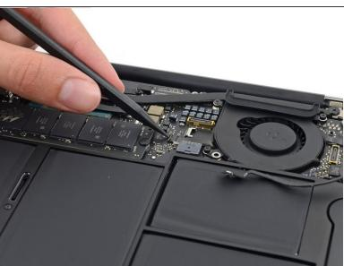
Use the tip of a spudger to carefully flip up the retaining flap on the fan cable ZIF socket.
