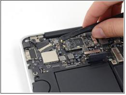
Use the flat end of a spudger to pry both antenna connectors up from their sockets on the AirPort/Bluetooth card, and move them out of the way.
