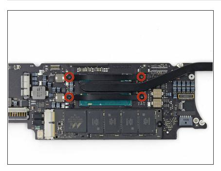
Remove the four 2.5 mm T5 Torx screws securing the heat sink to the logic board.
