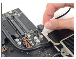
Disconnect and remove the SATA data and power cables from the logic board.
