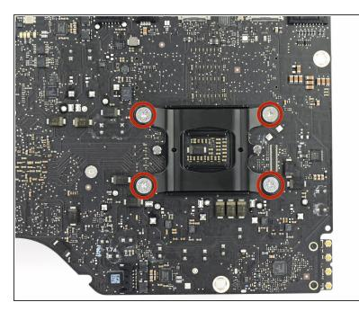
Remove the four 12 mm T10 shoulder screws from the spring plate behind the CPU.
