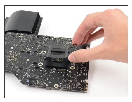
Remove the spring plate from behind the CPU heat sink.
