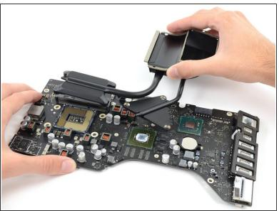
Lift and remove the heat sink up off the logic board.
